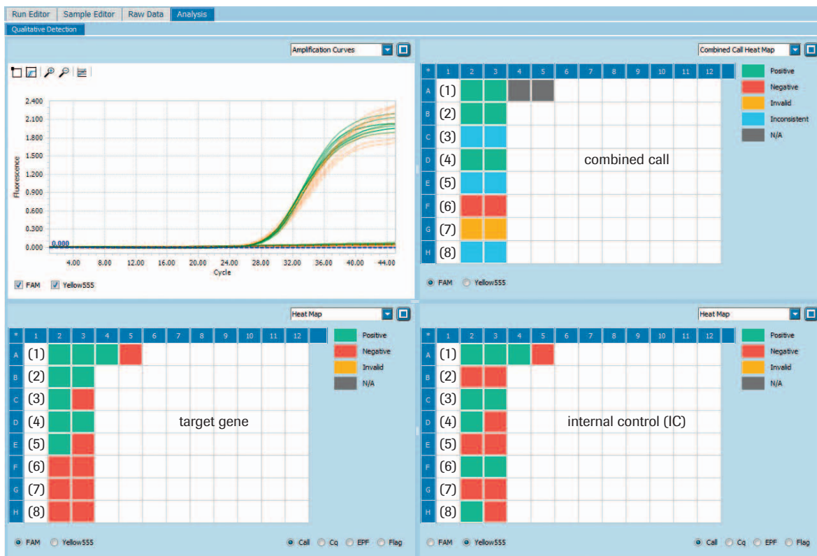
Figure 6: The Qualitative Detection Module provides a Combined Call by combining the individual calls of a target gene and an internal control (IC).
